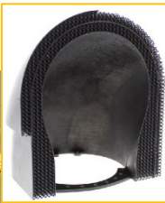
Helicopter exhaust gas nozzle with integral cooling. ( https://altairenlighten.com )
