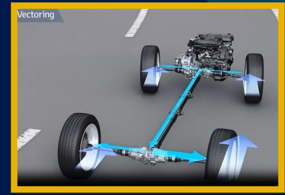
Control of vehicle dynamics through torque vectoring
